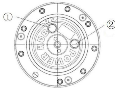
Figure 1-3 Traveling slowdown 1. Oil filler 2. Viewing port
