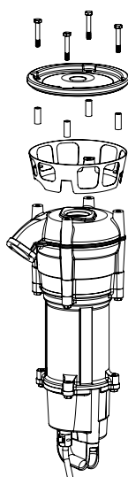
Figure 7a: Removing base plate, rubber sleeves and strainer
